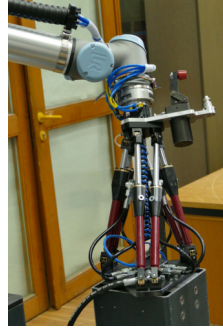
(b) The passive reconfigurable fixture being reconfigured by a UR10 robot.
