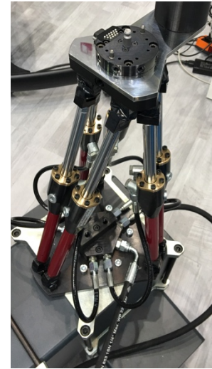
Figure 16: Hexapod reconfigurable fixture platform
