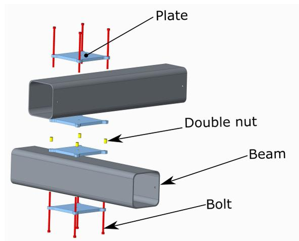
Figure 16: Double box joint structure
