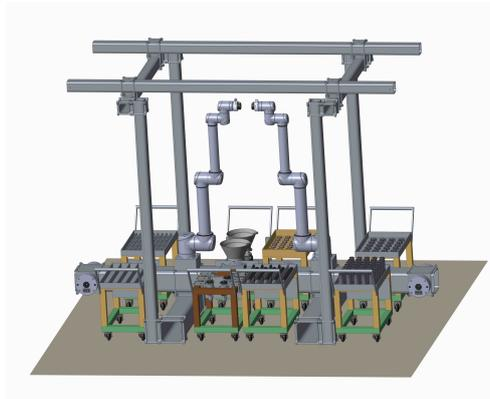
Figure 25: Final version of the LDT workcell design
