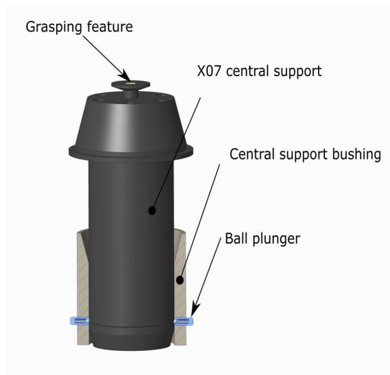
Figure 9: Exchangeable central support subassembly
