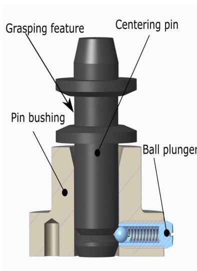
Figure 8: Exchangeable centering pin subassembly
