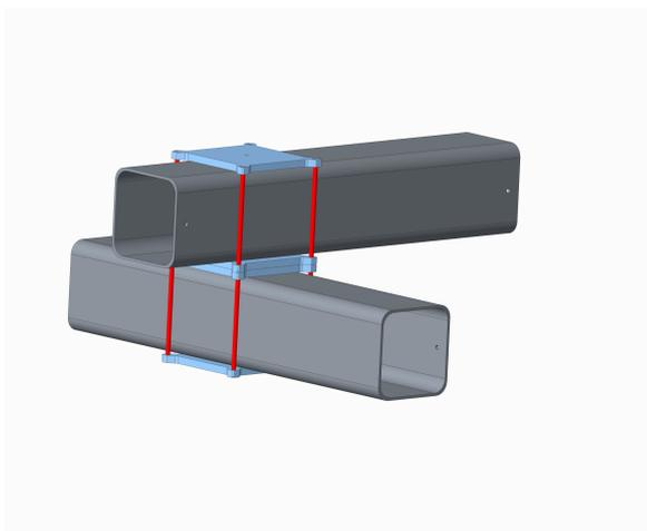
Figure 15: Double box joint
