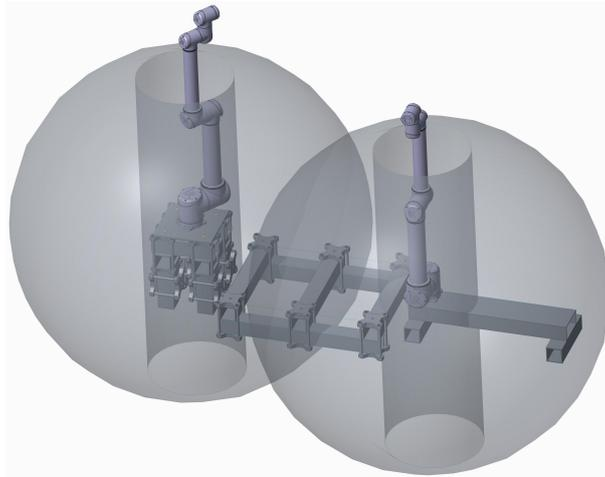
Figure 19: First draft of the ELVEZ workcell design.
