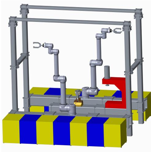
Figure 22: First draft of the PRZM workcell design
