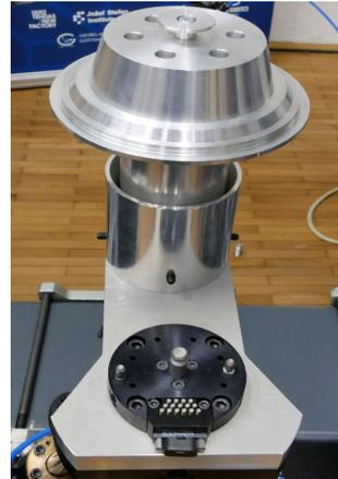
Figure 11: Light housing X82 central support
