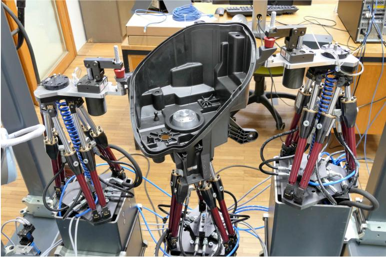
Figure 13: Reconfigurable fixtures for the ELVEZ use case
