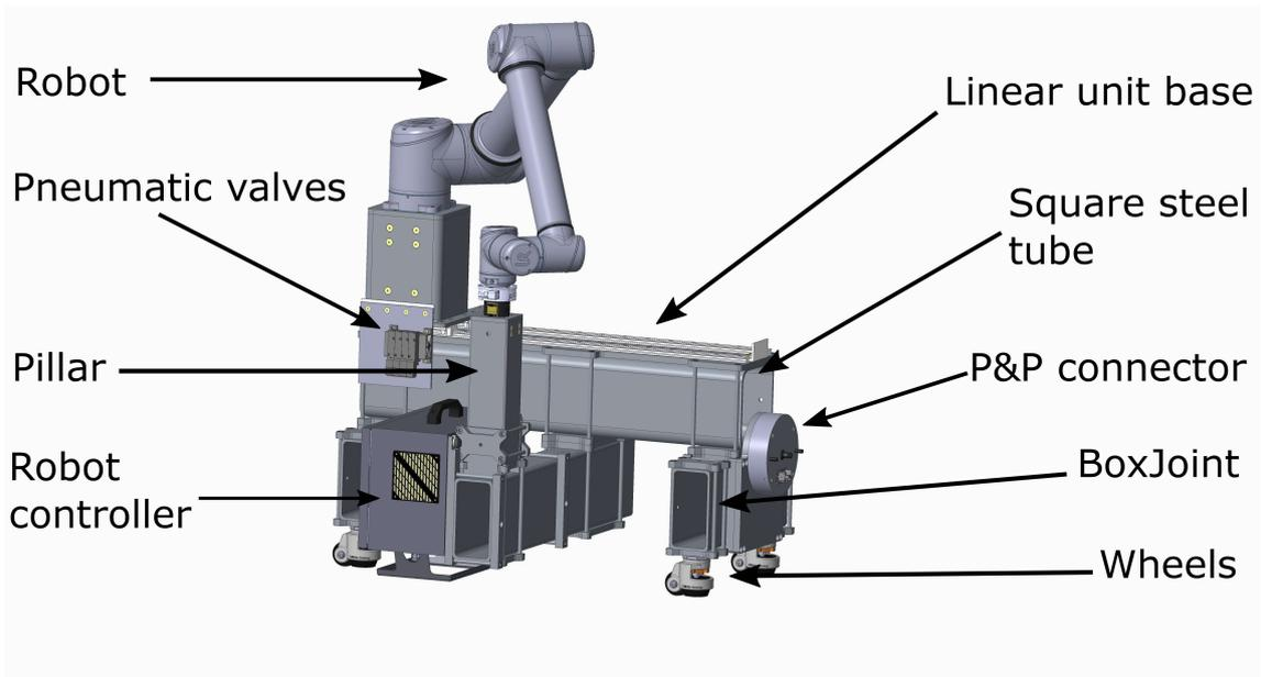
Figure 35: Integration of passive linear unit in the workcell
