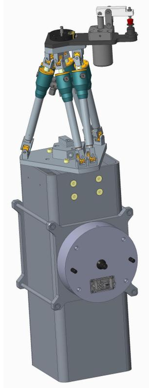
Figure 34: Reconfigurable jig module
