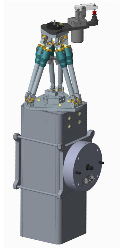
Figure 14: Reconfigurable jig module
