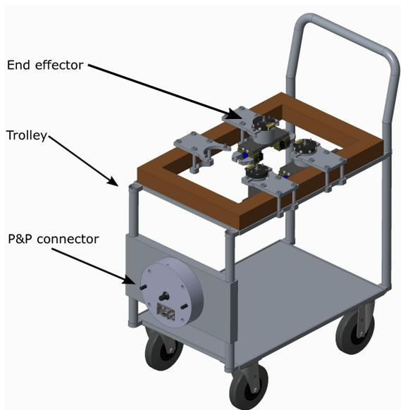
Figure 32: P&P tool hanger trolley
