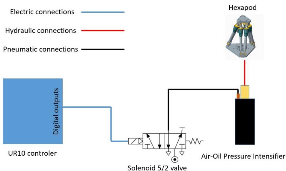
Figure 3: Schematic control diagram
