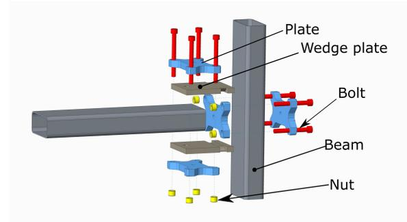
Figure 18: T-joint structure
