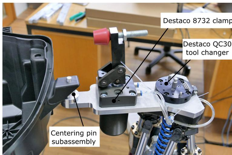
Figure 12: Hexapod mounted clamp subassembly
