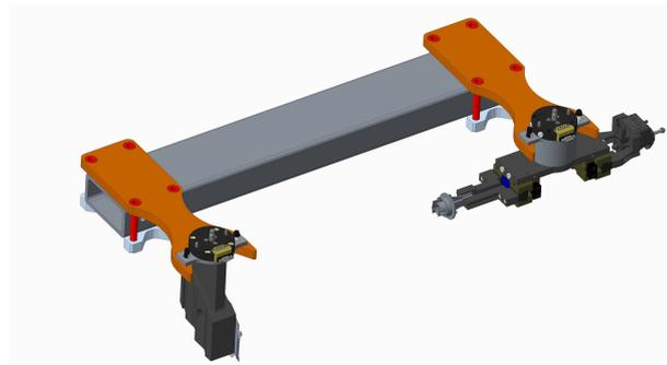
Figure 29: Two end-effectors stored on hanger modules
