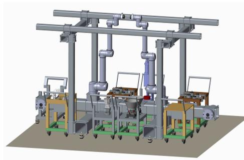
Figure 24: Final version of the PRZM workcell design
