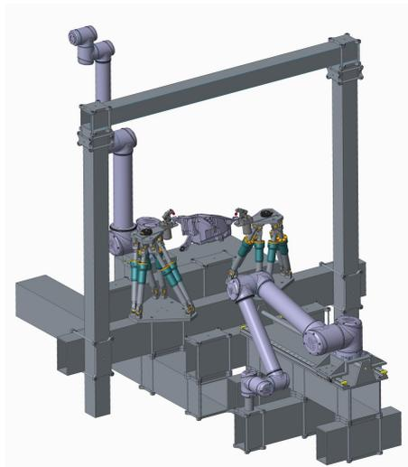
Figure 20: Intermediate iteration of the ELVEZ workcell design.
