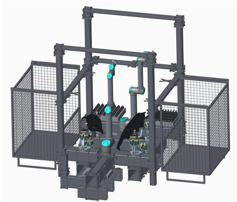
Figure 21: Final iteration of the ELVEZ workcell design
