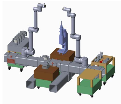
Figure 23: Intermediate version of the PRZM workcell design
